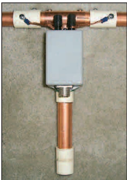
Figure 6 — Dipole feed connection — toroid balun option shown.
