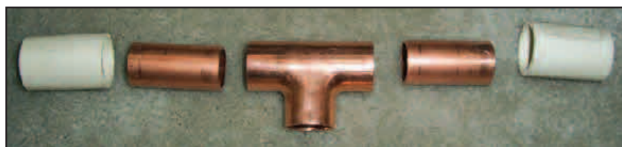
Figure 1 — Details of PVC and copper pipe pieces for antenna center.
