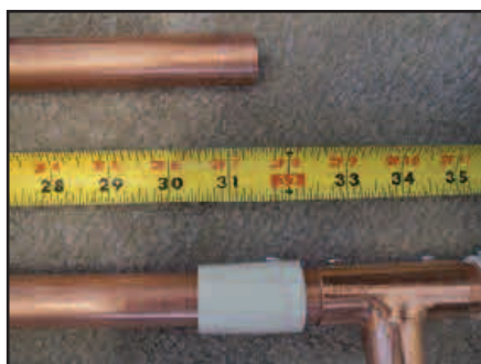
Figure 3 — Detailed view of inner element construction.
